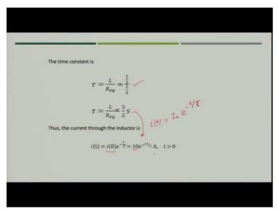
Now, what would be the value of time constant, time constant value will be L upon R equivalent value of L is given as 0.5 henry so that was given in the question so, we will put that value and the R equivalent we have just now calculated as 1 by 3 ohm so, value of tau will be 3 by 2 second, this value we will put in the original equation of current
