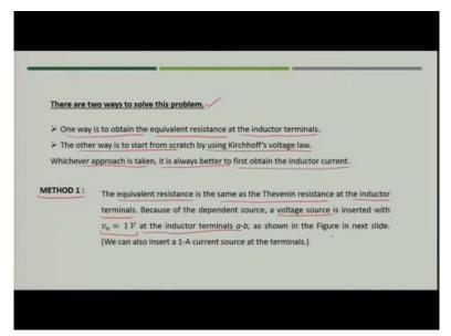
Now, here we have two ways to solve this problem, one way is that we can obtain the equivalent resistance of the inductor terminal, or other way is that, we start from scratch using Kirchhoff voltage law.
