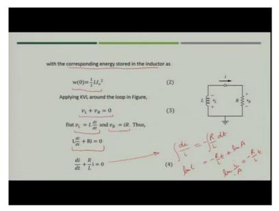
So, let us analyze the circuit. The energy which would be stored in the inductor initially is
