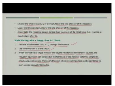
Now, let see some important facts about the time constant, smaller the time constant of the circuit faster would be rate of decay of the response. So, this is similar to what we saw in case of RC circuit so similar to that in RL circuit also the small time constant means faster the rate of decay of response.
