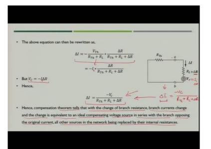
$$\Delta I = \frac{V_{Th}}{R_{Th} + (R_L + \Delta R)} - \frac{V_{Th}}{R_{Th} + R_L}$$
