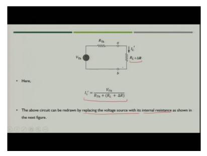
So, what happens now, the other parameters of the circuits are same. So, there is no change in the Thevenin equivalent, Thevenin equivalent will remain same, the only change would be the load resistance that is now  $R_L + \Delta R$ . Current now, flowing through the updated load resistors is now  $I'_L$ . So, what will happen, what would be the value of  $I'_L$  now,
