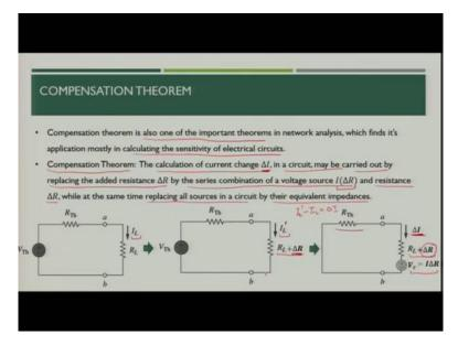
Now, let us talk about another theorem, which is called as a compensation theorem. Compensation theorem is also 1 of the important theorems in the network analysis, which finds its application mostly in calculating the sensitivity of the electrical circuit. Sensitivity means, when you change the value of voltage a little bit, say,  $\Delta V$ , how much the current will change in that particular segment, where you are trying to find out the sensitivity.
