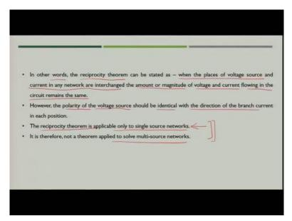
Now, in other words, you can also say that reciprocity theorem can be interpreted as when the places of voltage source and current in any network are interchanged the amount of magnitude of voltage and current flowing in the circuit remains same.
