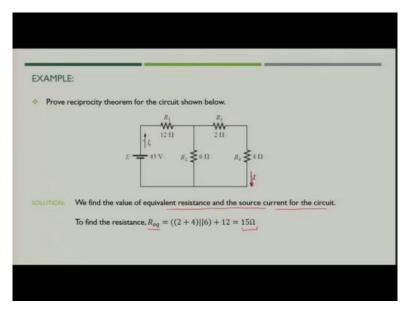
Now, let us understand this aspect with the help of an example. So, that you are clearer about the particular theorem. Let us see a particular circuit which is shown in this figure, we have a voltage source E that is 45 volt giving current as  $I_s$  to the circuit and the 4 resistance as you will see in the circuit are shown. Now, we have to prove that if you exchange the locations of I and E the values of current I is not going to change.
