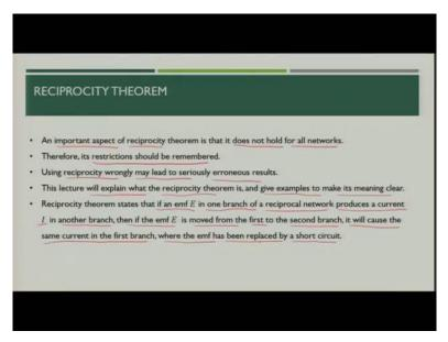
So, what does reciprocity theorem says basically. It is a very important aspect of reciprocity theorem that it does not hold for all network. So, we have to be very careful when we deal with the reciprocity theorem and we have to keep remembering the restrictions which are imposed on the reciprocity theorem because if you do not follow then the reciprocity theorem you will use wrongly and that may lead to a serious erroneous result in the circuit.
