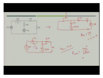
To find  $R_{th}$  you will simply short circuit this. You will get circuit like this in this case. So, this is dependent voltage source. This is  $3v_x$ , this is 1 ohm, this is 2 ohm and then you have 4 ohm and you need to find out the Thevenin resistance.
