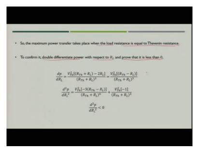
Now, as we discussed in the previous class, the maximum power transfer takes place when the load resistance is equal to Thevenin resistance. This we derived when we took the derivative of power p with respect to  $R_L$  which is variable and now, as we know that at the when the derivative  $\frac{dp}{dR_L}$  is equal to 0 at that condition. The  $R_L$  value what we get if you supply that value  $R_L$  into the power p power might be maximum or minimum.
