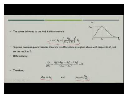
Now, we also discuss that, if you keep on changing the load, from 0 to infinity, there would be one point at which your power being absorbed by the load is maximum and that is the power being given to the load by the sources is maximum. So, that condition comes when  $R_L$  that is the load resistance is equal to Thevenin resistance and we stabilize that the power is nothing but  $i^2 R_L$  and we derived the maximum power transfer condition.
