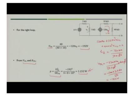
So, next what we have to do we have to find out the value of  $V_{Th}$ . So, here if you find out the value of  $V_{Th}$  what you get you will get again the voltage divider circuit or alternatively you can write the loop equation say  $i_2$ . This would be
