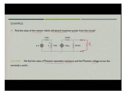
So, now, let us come to another example, where you will see there is one dependent voltage source available. Now, we have to find the value of resistance suppose if there is a load say  $R_L$  connected across the terminal ab. Now, we need to find out the value of  $R_L$  which will absorb maximum power from the circuit, that is the circuit which was given in the question. So, the load which will absorb maximum power from the circuit.
