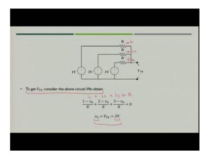
Now, next task is to find out the value of Thevenin voltage. Now, let us assume that the voltage at this particular node is  $v_0$ . So, what we can write we can use Kirchhoff's current law at this particular node and we will try to find out the value of  $V_{Th}$ . So, what you can right at this point for 1 volt what would be the current.
