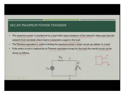
So, before going to the dependent source condition let us try to understand what we discussed in the previous class. We discussed about the maximum power transfer theorem, we said that the maximum power is transferred to a load when input resistance of the network, when seen from the terminal where the load is connected, is equal to load.
