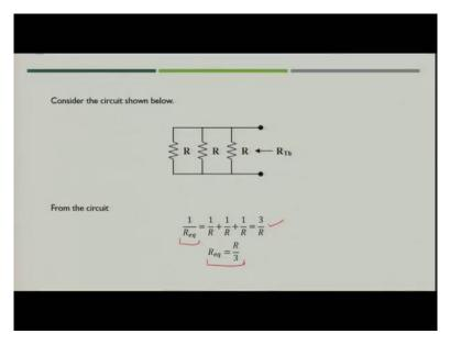
So, you will get this circuit as an equivalent circuit for after short circuiting all the voltage sources and then you need to find out the value of  $R_{Th}$ . So, here you will see all the 3 resistances are in parallel. So, what you can say if it is  $R_{Th}$  is nothing but  $R_{eq}$  across these 2 terminals. Then you can write
