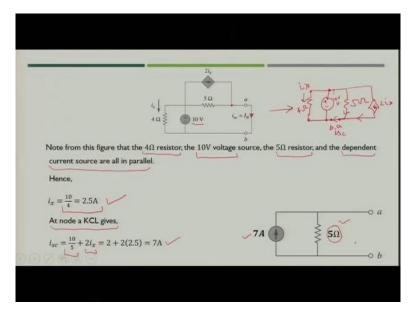
So, what we have to do we have to just short circuit the terminals ab. Now, we have assumed that there is a short circuit current  $i_{sc}$  which is nothing but the Norton's current and you have the circuit you need to find out the value of short circuit current flowing through short circuited terminal ab.
