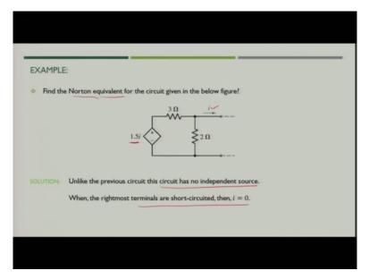
Now, let us see another case which is different from our previous example. In this case, we need to find out the Norton's equivalent, but the important thing which we see here that this circuit does not have any independent voltage or current source.
