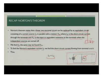
So, let us see the Norton's theorem which we discussed in the last class. Norton's theorem states that the linear 2 terminal circuit can be replaced by an equivalent circuit consisting of a current source  $I_N$  in parallel with resistor  $R_N$  where  $I_N$  is this short circuit current through the terminals and  $R_N$  is the input or equivalent resistance at the terminals, when independent sources are turned off.
