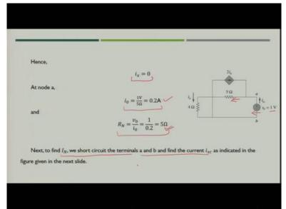
Now, what happens when  $i_x$  is equal to 0, you have this component 0, the current which is flowing from external voltage supply  $v_0$  would be only through the 5 ohm resistance. So, what we get the current
