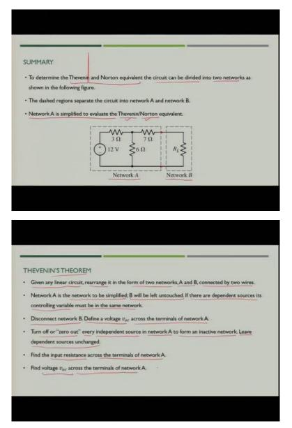
So, what we do in case of Thevenin's theorem. So, given any linear circuit, we rearrange it in the form of 2 networks A and B connected by 2 wires, network A is the network to be simplified and B will be left untouched. So, in this circuit, this would be simplified, then this would be untouched, if there are dependent sources, its controlling variable must be in the same network. That means if there is a dependent source in the circuit, the variable should also be in the same circuit.
