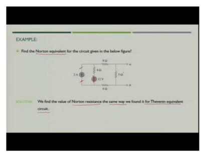
Now, let us understand the concept with the help of one example. So, the circuit which is given in the figure we need to find out the Norton's equivalent of the circuit. Now, we can also find out the value of Norton's resistance the same way as we found the value of Thevenin equivalent circuit that means what we have to do? We have to short-circuit the voltage source and open circuit the current source.
