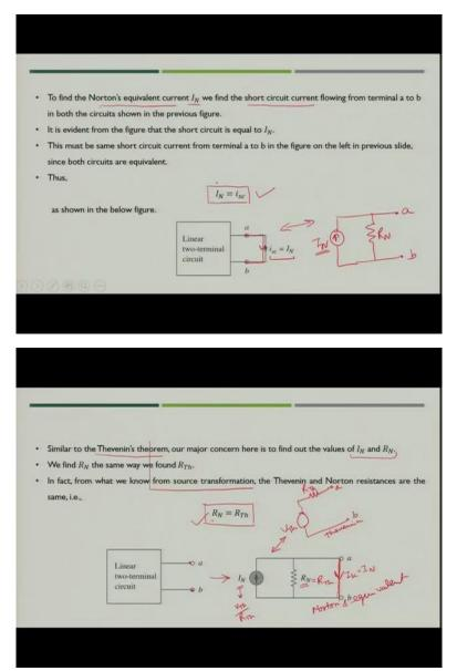
So, now the Norton's equivalent current how we will find out? We will find out while carrying out the short-circuit test on the network which is given to us. So, now if you see in this case if this is a two-terminal linear circuit we have to short-circuit these two-terminals and we have to measure the current that is short-circuit current. Now, when we find out the short-circuit current we will come to know that short-circuit current is nothing but the Norton's current, how?
