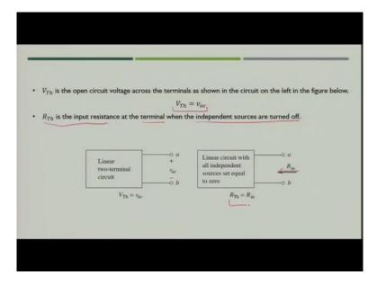
So, this is what we discussed in the last class and then we established that Thevenin voltage is nothing but open circuit voltage across the linear two terminal circuit and  $R_{Th}$  is nothing but the input resistance at the terminal when independent sources are turned off. So, if you look into the terminal a and b the equivalent resistance which you will see from here is nothing but the Thevenin resistance.
