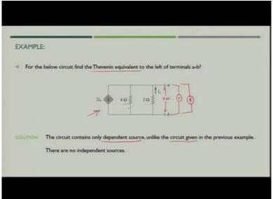
So, what we have to do? We just see that this circuit contains 2 ohm resistance in parallel with 4 ohm resistance so these two are in parallel and they in turn are in parallel with the dependent current source. Now, first thing which we have to consider is that since we do not have any independent source in the circuit we must excite the circuit externally, what does it mean?
