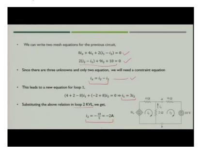
So, the updated circuit would be looking like this, here we have two meshes so what we have to do? We have to write the mesh equations for both of them so these would be the two mesh equations for these two meshes plus we will have another constraint for  $i_x$  that is nothing but  $i_2 - i_1$ .
