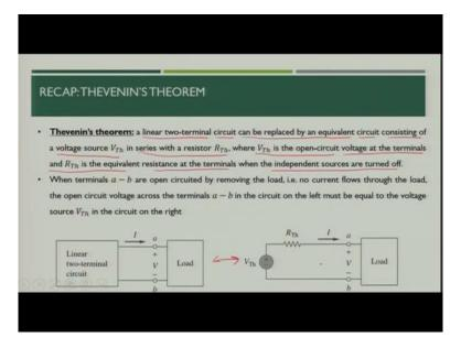
So, now let us start. First, let us recap what we discussed in the last class. We discussed Thevenin's theorem and we discussed that the linear two terminal circuit can be replaced by an equivalent circuit consisting of the voltage source  $V_{Th}$  in series with a register  $R_{Th}$  where  $V_{Th}$  is an open circuit voltage at the terminals and  $R_{Th}$  is the equivalent resistance at the terminals when the independent sources are turned off.
