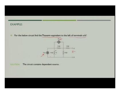
Now, let us solve it, what we have to do first? First, we have to solve for  $R_{Th}$  that is Thevenin resistance, in that case what we can do? We can remove all the independent sources, in this case this is a current source. You can make it open circuited. So, the resultant circuit would be like this and what we need to do is that? We need to add one voltage source  $v_0$  that is equal to 1 volt which would be connected across the terminals a and b and then solve the circuit.
