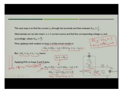
Now, what we have to do? We have to solve the circuit using mesh analysis. So, what would be the value of the mesh equation in case of loop 1? So this is loop 1 so when you solve since it is going from minus to plus across the dependent voltage source it will become
