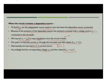
So, what the process we need to follow when the circuit contains a dependent source? We have to find  $R_{Th}$  that is Thevenin resistance we have to set the independent sources equal to zero and leave the dependent sources connected. Now, since the network has dependent sources we have to excite the network from outside with the help of either voltage  $v_0$  or maybe the current source  $i_0$  which would be connected to the terminals.
