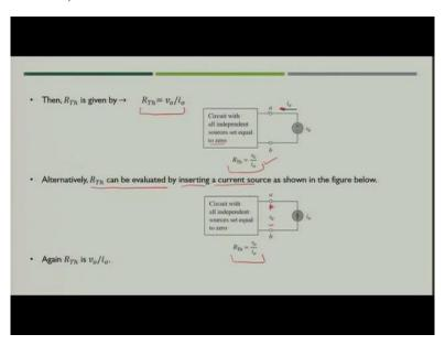
So, what does it mean? If you have circuit with all independent sources set equal to zero and the keeping all the dependent sources connected with the network, the terminal a and b would be supplied with voltage  $v_0$  which will supply some current  $i_0$ . So, in that case if you solve the circuit with the help of either Kirchhoff Voltage Law or Kirchhoff Current Law you will be able to find out the value of Thevenin resistance which would be nothing but  $v_0/i_0$ .
