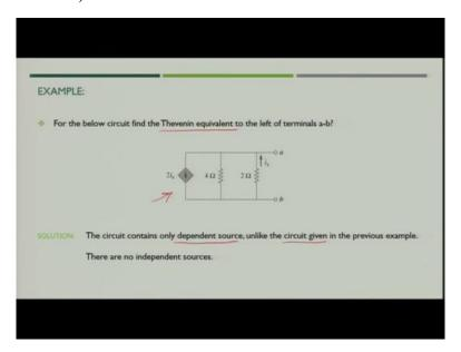
So now, let us see another example. In this circuit if you see the circuit we want to find out the Thevenin equivalent but in this particular circuit we do not have any independent voltage or current source, so the circuit would have only dependent source. So, here in this case we have the current source which is dependent.
