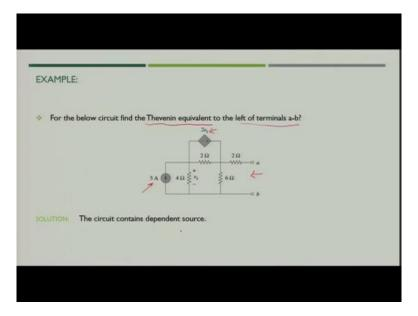
Now, let us understand this concept of how to solve the circuit when we have the dependent source with the help of one example. Now, let us see this particular circuit where you will see we have one independent current source of 5 ampere value additionally we have one voltage source which is dependent voltage source and the value of voltage is depending upon the voltage across 4 ohm resistance.
