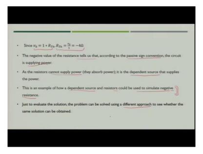
Now, since  $v_0 = 1 * R_{Th}$  because  $i_0 = 1$  ampere simply the value of Thevenin resistance would be minus of 4 ohm. Now, the negative value of resistance will tell us that according to the passive sign convention the circuit is supplying power. Since the resistor cannot supply power who will supply is this power? The dependent source which is connected to the network.
