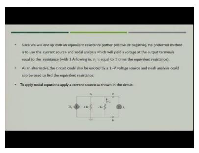
So, now let us apply one current source and try to solve it. Now, what we will do? We will see that this particular circuit has 1 node the voltage across this particular circuit a, b would be nothing but the voltage across both of the resistances also because all those elements are in parallel.
