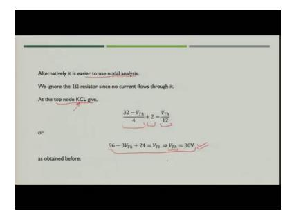
You will simply see what are the various currents flowing into the node and it equate it equal to zero because total sum of current at that particular node would be zero. What would be the current coming inside from left? That would be  $\frac{32-V_{Th}}{4}$ . So, you have got first term of the equation.
