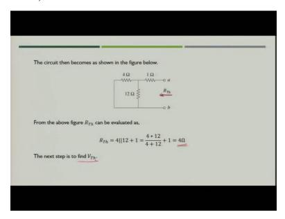
The resistance which you will see through these particular terminals that is a and b you will get the value of  $R_{Th}$  as 4 ohm because the parallel combination of these two resistances would give you 3 ohm plus 1 ohm in series. So finally, the  $R_{Th}$  value is 4 ohm. Now next step is finding out the value of Thevenin Voltage.
