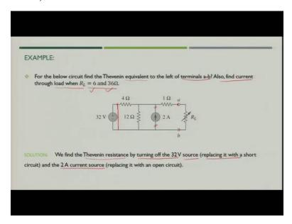
Now let us understand this particular aspect with the help of one example. Now you see there is a circuit given in this figure. We need to find out Thevenin equivalent to the left of terminal a-b. So, these are the terminals a-b and we have to find out the current through the load when  $R_L$  is equal to either 6 ohm or 36 ohm.
