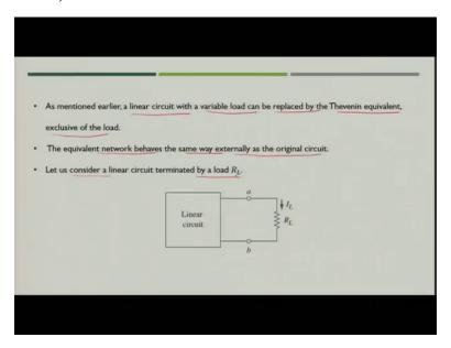
Now as we have discussed that linear circuit with variable load can be replaced by Thevenin equivalent excluding the load. Now this equivalent network will behave as same way as the external circuit is behaving, because you are creating the Thevenin equivalent of the external circuit by keeping vi characteristic equivalent.
