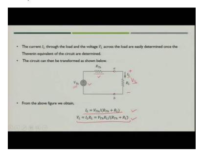
Now what you will do, the exact external to your load  $R_L$  would be replaced by its Thevenin equivalent that is  $V_{Th}$  and  $R_{Th}$ . So, what will happen in that case is  $R_L$  would be your load and there will be one resistance  $R_{Th}$  would be the Thevenin equivalent resistance and it would both would be connected through voltage source which is nothing but Thevenin Voltage.
