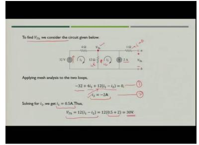
Now instead of Mesh analysis you can also apply Nodal analysis as well. So, if you apply the nodal analysis at this node because this is the node where you are seeing the voltage  $V_{Th}$ . If you apply nodal analysis that means that you have to use Kirchhoff's current law here. So, what will happen?
