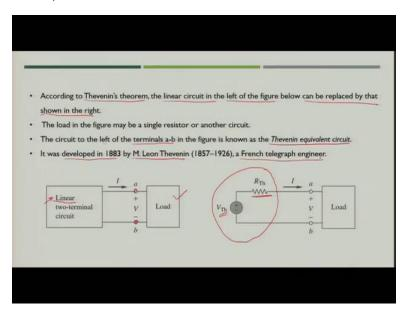
Now according to Thevenin's theorem, the linear circuit in the left of the figure can be replaced by that shown in the right. So, if you can imagine that these are the two points of your plug in the house. External to that you will see as a linear circuit. So, you have to keep in mind that the Thevenin's theorem works well when the circuit is linear.
