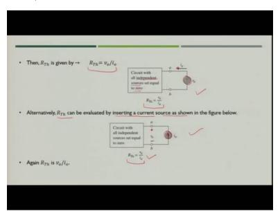
So, what will happen in that case? Here the circuit with all independent sources equal to zero are present. And the dependent sources are also available. In that case you have to apply one voltage  $v_0$  across the terminal of a-b and measure the value of current  $i_0$ .
