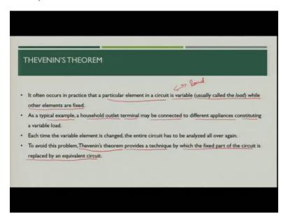
What happens when you plug in your appliance in the house. You will analyze the voltage and current parameters of that appliance, while neglecting the circuit which is outside the particular plug block plug point. So, what happens that you will analyze these circuit parameters like voltage and current while doing the analysis for various appliances.
