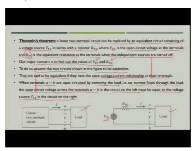
What does Thevenin's theorem says: A linear two terminal circuit can be replaced by an equivalent circuit consisting of a voltage source  $V_{Th}$  In series with resistor  $R_{Th}$  where  $V_{Th}$  is the open circuit voltage at the terminals and  $R_{Th}$  is the equivalent resistance at the terminals when the independent sources are turned off.
