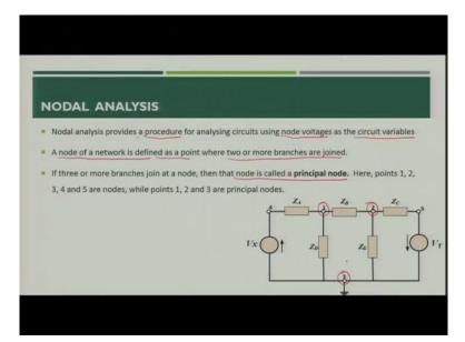
What do you mean by nodal analysis? Actually, nodal analysis provides a procedure for analyzing circuit using node voltage. So, in the mesh analysis we are more concerned about the mesh current and we were utilizing mesh current to solve the circuit. Here we will use node voltage as a circuit variable to solve the circuit. Now, node is the network node of a network is defined as a point where two or more branches are joined.
