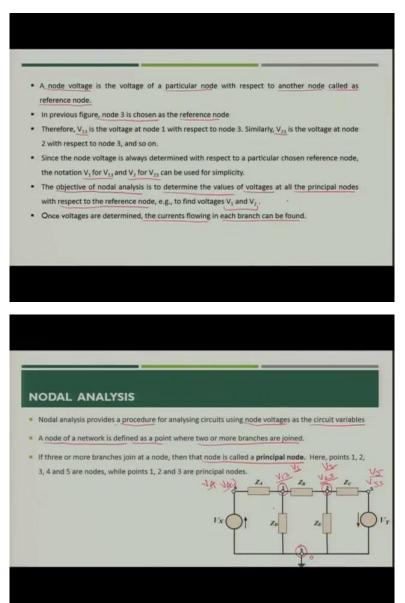
So, let us see what is the significance of the principal nodes. What is the node voltage? Node voltage is the voltage of a particular node with respect to another node which is called as a
