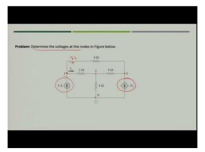
Now, let us take one another example in this case the node voltage needs to be determine but here the source is one is independent current source and second is the dependent current source. So, in this case when you have dependent and independent current source, how you will solve the circuit? You will follow the same procedure what we did in the previous example, you have to first find out the principal nodes.
