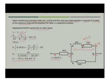
So, what you will do? You have to first find out the value of current  $I_Y = V_1/(4 + j3)$ . Now, we have to see what is the drop in this particular segment that is between A and B. So, what you will do? You will use Ohm's law and whatever the current is flowing that is  $I_Y$  and multiplied by the resistance 4 would be the voltage at node A.
