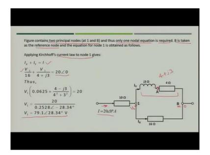
So, how you will solve? You have to again find out the principal nodes, so what are the principal nodes? The principal nodes here are 1 and B because these are the only two nodes where number of branches connected at three, so you have got principal nodes. Now, out of that only one nodal equation is required because you have taken B as a reference node. So, you need to write only one equation to solve the voltage at node 1 that is  $V_1$ .
