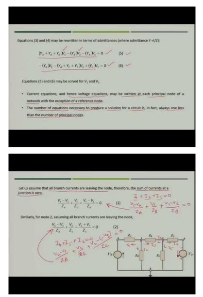
So, what you can write now? You can simply write the equation in the form of admittances and the now you have simpler equations you can solve it for unknown variables which are  $V_1$  and  $V_2$ . So, you have two unknown variables and two equations which can be easily solved. So, the current equations enhance the voltage equations may be written at each principal node of a network with exception of reference node.
