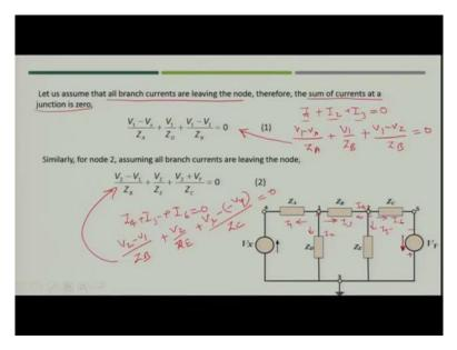
Now, how will we carry on this particular operation? Let us assume that this is the circuit which we saw previously and we will apply the nodal analysis and try to find out the values of node voltages  $V_1$  in  $V_2$  and then accordingly you can find the voltages and currents for say that is  $V_5$  and  $V_4$  and the currents flowing in the branches. Now, let us take the first node that is node 1.
