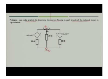
So, you have got the value of  $V_1$  simply you have to put the values of  $V_1$  in  $I_1$ ,  $I_2$  and  $I_3$  and when you will put the value you will get the values of currents, right. So, in this way you can easily find out the value of currents of those are the branch currents in this case and you can solve the circuit.
