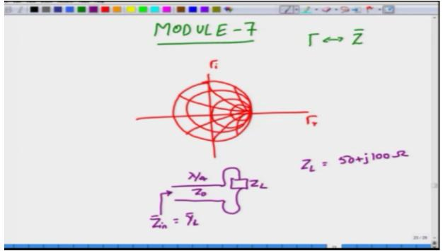
so if you want to un-normalized it you simply multiply admittance which is normalized with Y0 which is your admittance of the transmission line, okay.
