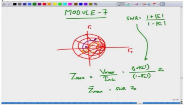
Normalized Z max is exactly equal to SWR, okay, you can in fact show that normalized Z min that is impedance will actually be equal to 1/SWR, now you don't have to do any other
