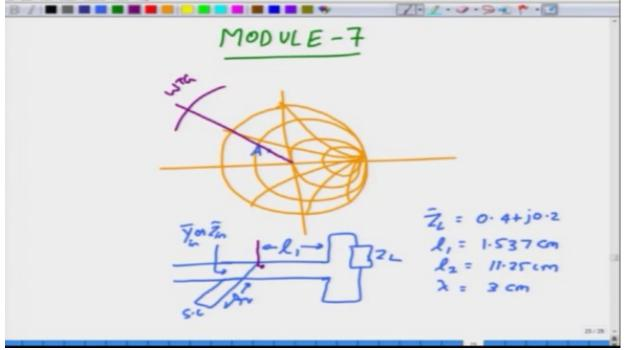
So after locating here and after drawing a line and extending it on to WTG scale and noting down the points over there, now I also want to draw a constant SWR circle, okay which is obvious, so specify this constant R equal to 1 circle with a different colour, because this circle will be very special for us, so always draw slightly thicker circle on this R = 1, so that you are now working with that.
