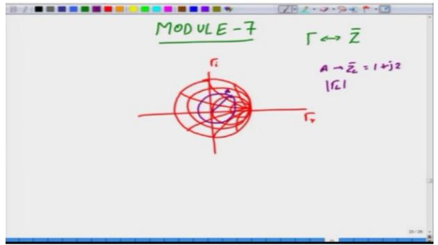
in fact commercial Smith Charts actually have a scale given down, okay, which will you know indicate both magnitude as well as angle, so there will be magnitude gamma L as well as the angle theta gamma in degrees, okay, so you simply take your compass measure this length here from 0 to A, and then cut that on the two axis, read the value here you will get gamma L and you will also get theta gamma, okay, so this is as simple as that, (Refer Slide Time: 12:44)
