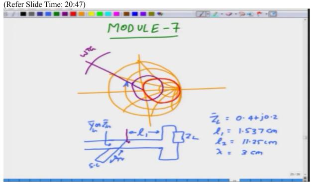
Now what you have to do is to move from this load point all the way up to L1, right, I mean a distance of L1, but because of the transmission line you are going to move distances relative to
