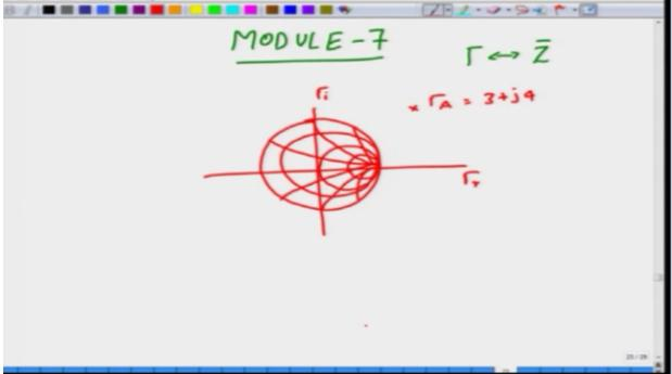
and because there is a one to one relationship between this one and the normalized impedance you can also calculate normalized impedance from gamma, right, you know how gamma is
