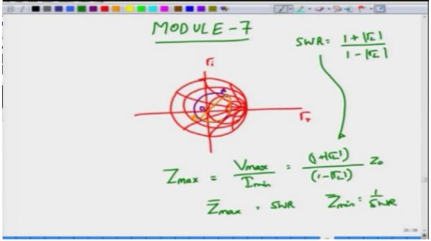
so when you cut the real axis here that would be the point where you will get the maximum value of small r, which is basically the normalized maximum resistance which is also equal to SWR, so in one point you actually killed 2 stones, right, you killed 2 stones with a single bird normally you kill 2 birds with a single stone, now you did the other way around and what you did or what you obtained was both information on Z max as well as SWR, okay.
