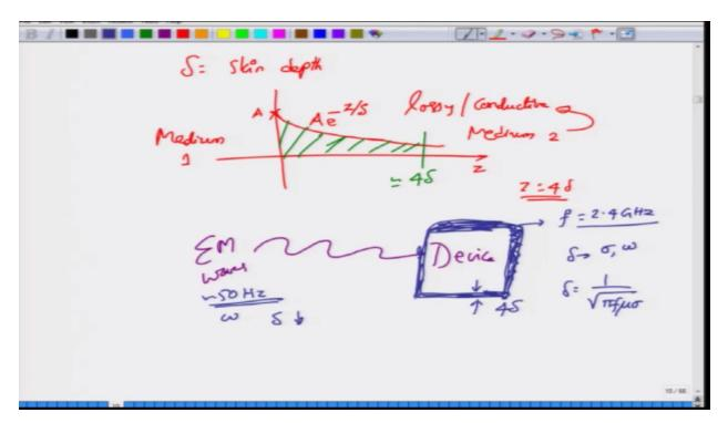
This  $\Delta$  is a very important parameter called skin depth. This is called a skin depth meaning that if we launch an electromagnetic wave into a completely
