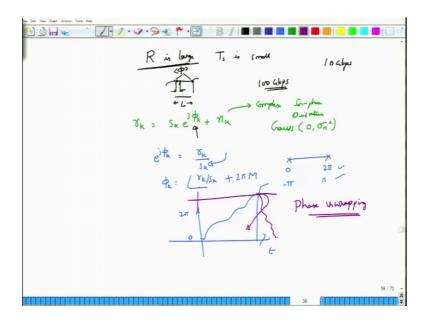
When R is large, T s is small which means the samples that are being taken are much more closer to each other and there is sufficient correlation between those samples when you take them to be very close with respect to each other.
