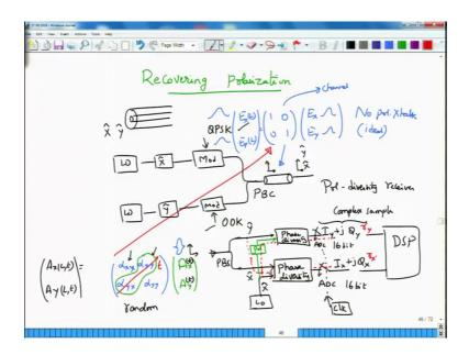
It is important to recover the polarization because in most optical-fiber communications today, we use both the x as well as the y polarizations in order to transmit information. So, usually what we have is y information source which produces or which produces x polarized light. And then you can modulate the data onto this one using an external modulator as in a usual sense and then combined this one with another laser output which is polarized along the y direction ok.
