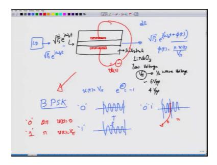
So, if we look at the integrated moderator structure you would see something like this. This is the substrate which is an electro optic substrate and the most popular electro optic substrate which has this large bandwidth, high electro optic coefficient and an appropriate voltage value of studies you know you can modulate. But, if your voltage requirements are like say 100 volt, 200 volt then it makes no sense, right. But, these
