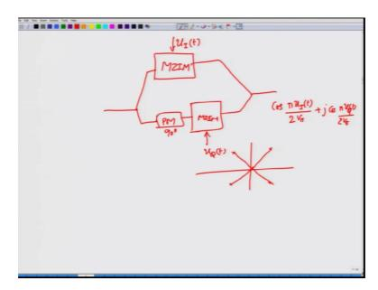
Then there is another device called as IQ modulator. In this IQ modulator what you do is that you actually have MZIM in one arm, ok. You send out the input light is split into two parts. So, you have a phase modulator which is configured to provide 90 degree phase shift and then you have one more MZIM and the signal to this MZIM will be together called as u I of t and the signal to this one will be called as u Q of t and then you combine these two outputs onto a output coupler.
