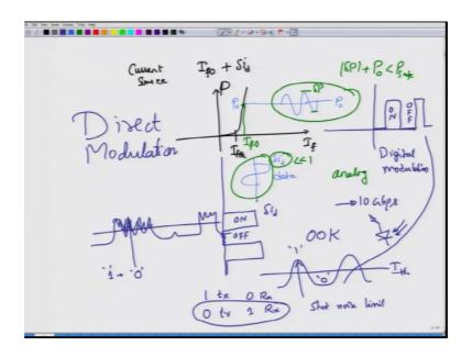
So, I can put the current source to generate some constant value which I will call as say I f 0 and I f 0 would be the bias current that is necessary to sustain the lasing action of the semiconductor laser diode and any data that I want to transmit I can actually put that data as or superimpose that current onto the forward bias current.
