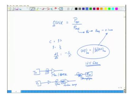
Associated with this erbium doped fiber is one last term that will come up very importantly in the cases when we discuss communication systems. So, when we start doing that it is called optical signal to noise ratio. That is if we were to able if we were able to directly measure whatever the optical power that is present in the signal, and then take the ratio of the total average noise power then this is called as optical signal to noise ratio.
