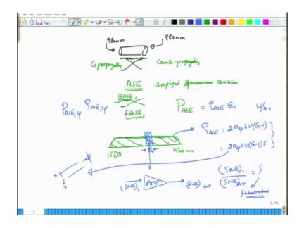
This also indicates another idea that one can use. While the forward pump drops down is it possible for us to actually use a secondary pump and in the backward direction while the forward direction pump starts off initially being very strong, and then eventually falls off. What if we could actually have another pump in the backward direction which could then start off strongly here and then go down as it goes?
