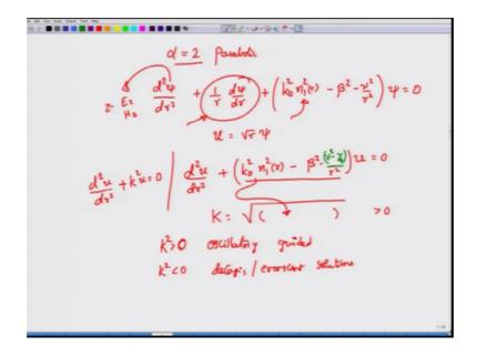
And that special case happens to be what is called as parabolic grading or parabolic index profile, because for that case alpha is equal to 2. In a certain approximate sense, the equation that you will be solving would look something like this, the where psi corresponds to the z component of the electric field or the magnetic field. So, this would correspond to E z or H z have denoted that one by just using this psi.
