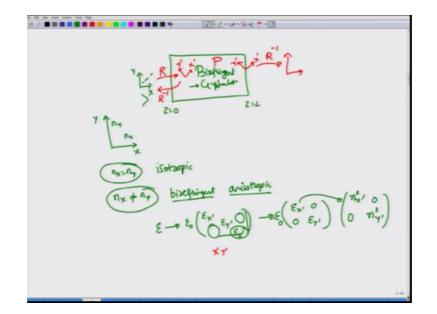
So, how do we go about understanding this PMD, well to understand PMD we need to first understand how light propagates in the so called birefringent medium. Now, what is birefringent medium? Well, you know if you go to simple X and Y coordinate system, and you have a pulse which is propagating along the z axis ok..
