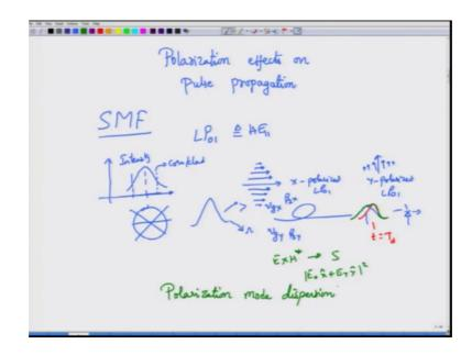
What do we mean by polarization effect on pulse propagation? What we mean is well, let us focus our attention only on what is called as single mode fiber which means that we are dealing with only one mode at a given operating range.
