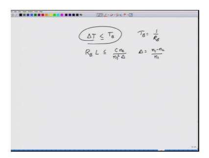
And this pulse broadening eventually have to be in such a way that, you the pulses broadened by less than say amount of T B which is the pulse, or the bits slot that I am sending out. So, if this delta T is less than or equal to T B, then 1 I mean this is one criteria of course so, if I let that the pulse broadening be less than the time slot, or equal to 1 time slot, then I will be able to communicate at this particular rate ok.
