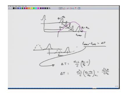
So, I being at no 0 or at whatever the time which is taken minimum time of arrival as measured from 0 axis and, then you have another one which is arriving ok, with the max angle of or with the max time of t max. And there will be all this intermediate pulses so, corresponding to different angles of theta 1 between this is for theta 1 equals pi by 2 and this for theta 1 equals theta 1 c, for all angles between them they would all be arriving at different times which are between t min and t max.
