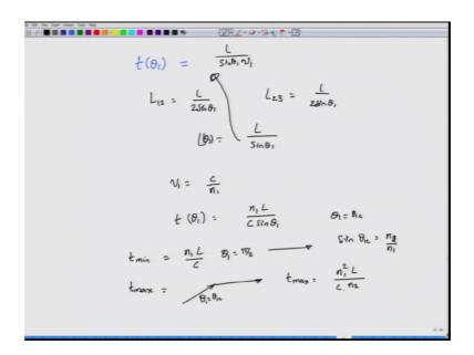
And the velocity with which for the time delay that is now taken by this ray of light, which is actually making an angle of theta 1 is given by L 1 to sin theta 1 plus L two 3 sin theta. So, this one is sin theta so, this is L 1 2 sin theta 1 L 2 3 sin theta 2. So, for the ray that you know is given by this blue line, if I assume that the distance between 1 2 3 is L.
