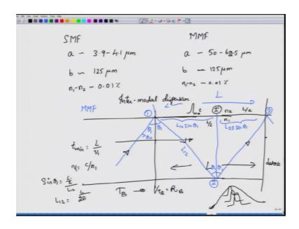
For standard single mode fiber the core radius a goes anywhere between 3.9 to 4.1 micrometre the cladding radius b is usually standardise to about 125 micrometre ok.
