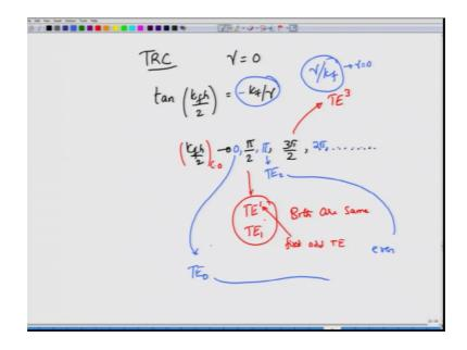
So, if you look at the transverse resonance condition that we derived for the odd mode and for the even mode and for the odd mode it is a reasonably simple way to derive that one which we will do it later. So for the transverse resonance condition if you look at that and then demand that for cut off; since gamma must be equal to 0 for cut off what are the different values of kappa f and hence what is the different values of beta that you would find?
