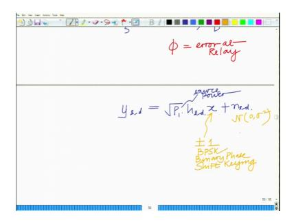
Now, let us try to model this link. This link can be modelled as the received symbol y corresponding to transmission by the y s d, because this is the source destination link, equals well square root of P 1. Let us assume that the source transmits with power P 1 square root of P 1, this is the source power times h s d channel. We have already seen this, this is a flat this is the fading channel coefficient between source and destination times x, which is the transmit symbol plus n s d.
