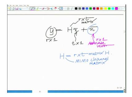
And our model for this MIMO system is therefore given as y bar equals H x bar plus n bar where we know this y bar this is an r cross 1 receive vector, this is a t cross 1 transmit
