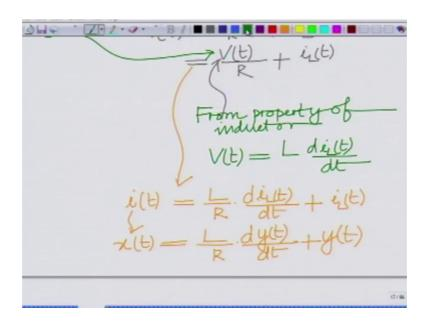
So, I finally, have x of t equals L by R; d of now i L of t is y of t that is output. So, this is d y t divided by the d y t with respect to d of t that the derivative is that is the, so L by R d y t over dt d y t or d y t dt plus y of t. And this is basically your input output relation or basically you can write it as L by R d y t; dt plus y of t equals x of t.
