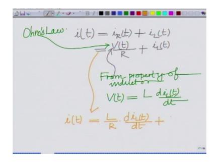
So, I have; well, firstly you can observe that by Kirchhoff's current law you have i of t; that is the current of the source i of t is the current in the resistance plus the current in the inductance. So, that is simply by KCL; Kirchhoff's current law. So, I can write i of t equals i of R t plus i of L of t.
