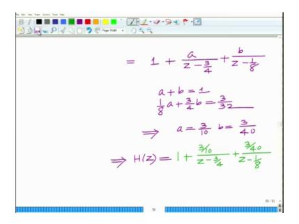
And now let us expand this into partial fractions, we can quickly do this. Let us say this is equal to 1 over z minus 3 by a over z minus 3 by 4 plus b over z minus 1 by 8. You can see that the coefficient of z; a plus b equals 1; further coefficient of z or negative a coefficient of the constant; 1 by 8 plus 1 by 8 a plus 3 by 4 must be equal to. So, minus 1 by 8 a minus 3 by 4 b must be equal to minus 3 by 32 which implies 1 by 8 a plus 3 by 4 b must be equal to 3 by 32.
