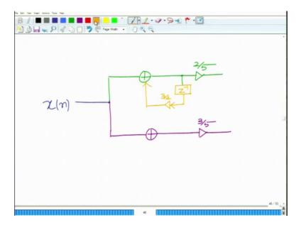
So, this will have 2 branches the top branch will be corresponding to the first factor that will be 2 by 5 by 1 minus 3 by 4 z inverse. So, that will have a gain that is 2 by 5 and
