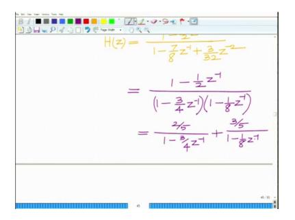
So, this is the partial fraction. So, these are the factors in the partial fraction expansion. And you can see each of these is a first order fraction; first order factor in the partial fraction expansion all right and now we are going to illustrate the PF 1; that is a the parallel form 1 structure for this IR filter ok. And therefore, it is very simple now you can see it has 2 factors. So, we will have 2 branches.
