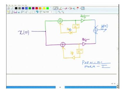
And this is your delay z inverse and this is the gain 1 over 8 ok. And therefore, now what we have is we have to add the outputs of both the branches. So, we have an adder and the output will be y of n ok. So, this is basically your parallel form 1 ok. So, this is the parallel form 1 ok. So, this is a parallel form 1 structure for the IR filter. So, this is 3 by 4 correct.
