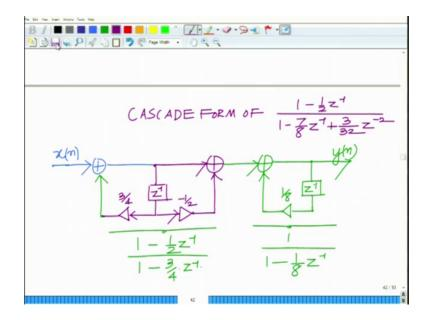
So, we have this, your x of n all right and that will go here you have a delay. You have a delay z inverse and here you have the gains that are basically minus half and here you have the gain that is 3 by 4 and that is going inside the adder correct ok.
