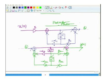
And this can be represented as follows: I have x n, cascade of one system after the other. So, x n let us put it this way goes through gained P naught correct and then we have z inverse and we have the adder over here and this will go to another gain this gain will be beta 1 corresponding to the numerator. So, we will go to the adder. We have another gain minus alpha 11 where alpha 11 is a coefficient in the denominator all right.
