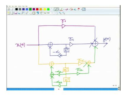
And the structure of this parallel form this can be given as follows. So, you have x n. So, now we will have these parallel branches. So, you have the first one that is the gain gamma naught then you have the gain gamma naught 1 and this is y n and here you have the delay z inverse and you have minus alpha 11, this is the DF 1 representation of the first term and then you will have the second order factor.
