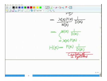
So, I can write this as W z into 1 over D z Y z equal to W z into 1 over D z where, W z equals X z into P z. So, this is a cascade of 2 systems that is P z into 1 over D z. So, H z is the cascade of these 2 systems ok.
