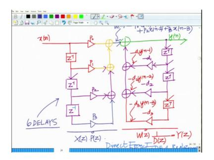
So, previously what you see is we had here we are DF 1 notice we had 6 delays ok. So, notice here we had 6 delay elements all right. So, there are 6 delay elements here and from this 6 delays what we have here is we have only we have managed to reduce this to basically 3 delays.
