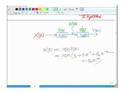
Now, let us look at, so I have Xz given as input to the first system; H1 z, the output Wn is given as input to the second system H 2 z and this is Wz and the intermediate signal is given by the z transform Wz. So, H1 z is basically your Pz and this is your 1 over Dz ok.
