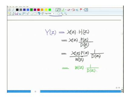
I can write this Y z equals X z into X z which is X z into P z divided by D z and this is X z into P z into 1 divided by D z. So, I can call this implement this as a cascade of 2 systems; I can call this X z into P z this can be defined as W z.
