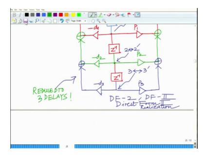
By fusing them suitably so what we have managed to do is we have reduced it to, so reduce the delays by a factor of 6. We have come down to 3 delays already. That is the advantage of the direct form direct form 2 realization all right. So, in this module we
