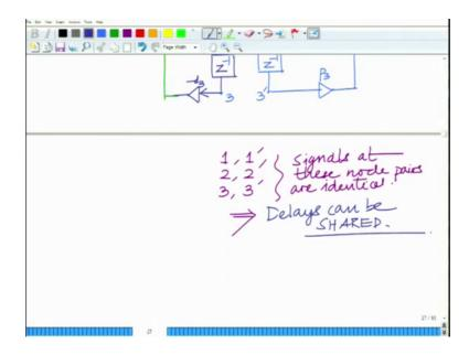
Now, these pairs are basically signals. This implies the signal that these node pairs are identical. This implies that you can delays can be shared; implies basically those signal points can be merged. So, delays these delays can be shared in a common.
