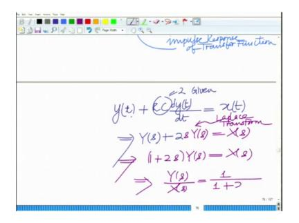
and we have seen this several times before yt is the voltage across the capacitor plus from ohms law R into I that is C dv by dt or C dy t by dt; that is the potential drop across the resistance and this has to be equal to the input voltage that is xt, which implies that y of which implies that now taking the s transform Y of s plus RC and RC we know equals 2. So, Y of s plus 2, so given RC equal to 2. So, given this RC equal to 2 that is given ok
