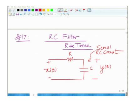
So, let us proceed to the next problem that is problem number 17 and this is with respect to an RC filter and this blocks talks about the rise time of an RC filter. And this deals with the concept of the rise time of an RC filter and the problem is as follows. So, let us say we have a serial RC circuit; we have a serial RC circuit, the output across the capacitor the input is the signal xt and the output across the capacitor the output voltage across the capacitor is yt.
