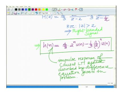
Which implies that this quantity h of n that is impulse response h of n is simply 4 by 3, 2 raise to n u n minus 1 by 3 of course this is z over z minus half, minus 1 over 3 times half raised to n un that is basically your impulse response of the LTI system described by the of the causal LTI system described by the differential equation given in the problem all right.
