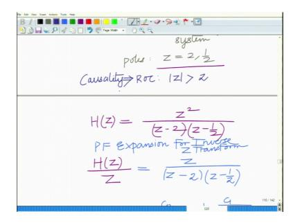
Now also H z now remember H z equals z square by z minus 2 so, the poles are z equals 2 comma half, because we can write this as now H z can also be simplified as observe z square over z minus 2 into z minus half. So, there are 2 poles at z equal to 2 and z equal to half, these are poles each pole has multiplicity 1 all right. So, these are simple poles and the poles are z equal to 2 and z equals half ok.
