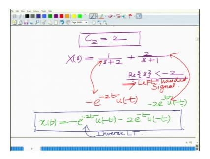
When ROC is of the form real part of s less than sigma max; so this will be of the form minus e raise to minus 2 t u minus t this is of the form that is the time domain signal corresponding 2 over s plus 1 is minus 2 e raised to minus t u minus t therefore NET signal x of t, will be minus e raise 2 minus t or let me just write it clearly x t is minus e
