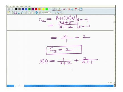
And therefore, C 2 equal to 2 and therefore, from the partial fraction expansion we have X s equals 1 over s plus 2 plus 2 over s plus 1, now you can see the ROC is real part of s less than minus 2, which basically implies that it is a left handed signal ok.
