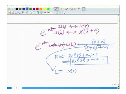
Now, remember we have the property recall we have the property e raise to minus a t x t has the Laplace transform x of s plus x of s plus a correct. So, where X s is a Laplace transform, that is if x t has the Laplace transform X s correct, then e raise to minus at x t has a Laplace transform X s plus a therefore, e raise to minus a t cosine omega naught t u t will naturally have the Laplace transform s plus a that is replace s by s plus a s plus a whole square plus omega naught square.
