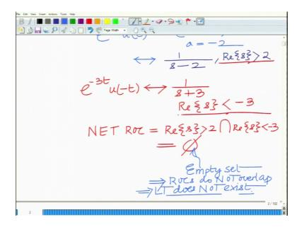
So, this intersection correct this intersection equals phi which is basically empty set correct, this is the empty set implies that implies basically ROCs do not over overlapped implies that Laplace transform exist does not exist for this signal.
