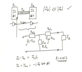
Then lambda Line circuit works very well when the transmission line length is very small compared to the wavelength of the source that you are connecting we are connecting. coming back if I consider lengths of point zero five lambda here I can find out what would be  $\beta$  Redcap
