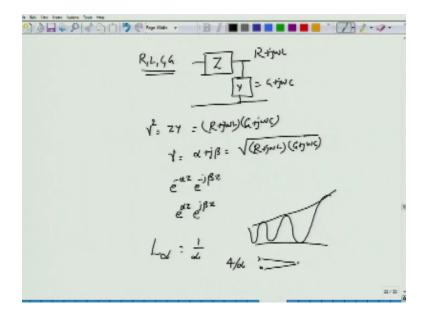
We consider the more general transmission line wherein we had rlc and g all terms related to the transmission line where present it resulted in the transmission line having a units cell with the series impedance and a conductance or the admittance of y, y was given by  $g + j \omega c z$  is  $R + j \omega l$ ,
