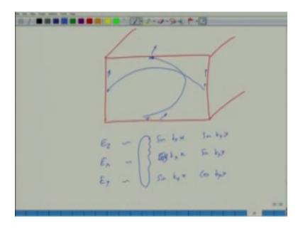
So this is the cross section of a wave guide right, if I am looking at Ey component where I want both Ey to be function of x and y and Ex component to be function of x and y, as well as Ez component for example if I am looking at the TM mode I need to know what is the Ez component as well, right. How do I write down the form of the solutions without actually solving Maxwell's equation.
