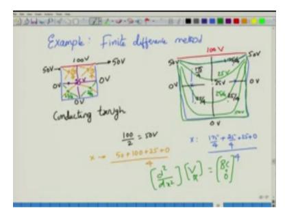
So let me redraw this one so this is slightly bigger picture that I am going to draw okay and then I have the top conductor which is kept at 100v and I have 50 v at the gab 50v at the gab at the
