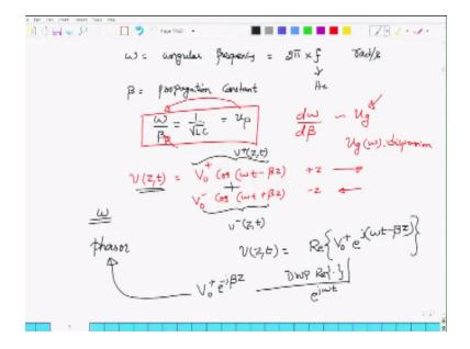
So this is the meaning of what we call as the phase velocity and it is the ratio of  $\omega$  to ß that determines what is the phase velocity and in this particular case it so happens that this ration omega/ß is given by  $1/\sqrt{LC}$ , okay. So this is something that you should remember we will later on see that the ration D  $\omega$ /D ß which tells you how the velocity itself is changing will be the one that will decide what is call as the group velocity.
