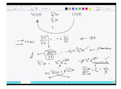
Now let us get back to an interesting thing we know how to obtain the voltage as a function of Z and T on the transmission line we also know how to obtain the corresponding you know phaser's V + (Z) or V - (Z) or V0 + (Z) or V0 - (Z) can I actually obtain what is I (Zt) from the voltage it should be possible for us to do so right, I should be able to obtain what is the current from the
