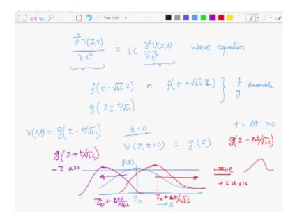
If you recall what those equations are that equation tells you on the left hand side how the voltage would be changing, voltage being a function of both Z and T on the transmission line. So on the left hand side of the equation you have the voltage changing as a function of Z remember Z is the axis along which the voltage or the axis of the transmission line that we have considered.
