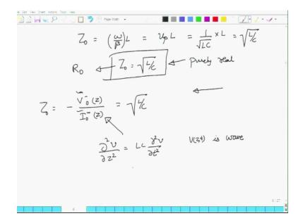
What is  $\omega l/\beta I$  can simplify this further because I know the relationship between  $\omega$  and  $\beta$ . So I have  $\omega /\beta x l$  is nothing but where the phase velocity x l up the phase velocity given by 1/le for this particular loss vision vertical line this one l/c. So the Characteristics Impedance of this transmission is purely assuming that both l and c are real and r and c are positive.
