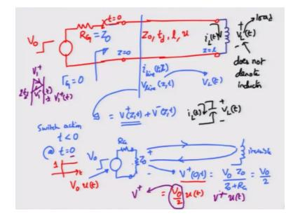
Remember we had a source somewhere right this source we had considered to be a step kind of a source we are considering the idealized step voltages the amplitude of the step voltage let us say is equal to V0 and this was connected via resistance or the internal impedance of the source which we called as RG in the previous module we let RG to be whatever the value it was and therefore there was reflections at the generator side as well.
