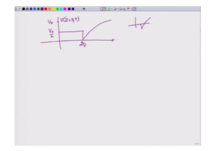
You can draw the voltage at the load side and that load voltage will be initially an amplitude of v0 / 2stepis propagating and when you receive now a voltage of the form this way initially negative and then going towards positive that step would be equal such that the you know enquiring magnitude but opposite in sign 2 v0 / 2 such that it will pull down the voltage completely to 0 at this point and then begins to raise to a final or in assume total value of v0.
