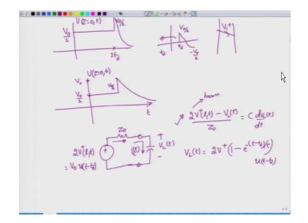
So outgoing voltage at if I along want to plot that total generator voltage at Z equal to 0 I know that I am already sending V0/2 this V0/2 is the initial V1+that we have right so this v0/2 is travelling at a time of 2 times of too time delay the reflector voltage which would be off this for me started of in this way at time t=td would now arrive after the time delay of td seconds.
