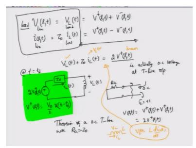
So at t= td and thereafter we know that line voltage that we considered let us call this as some v(l, t) where v(l, t) will be the total voltage I have dropped the subscript line here into this one I have dropped the subscript line here and this is the load side voltage correct, so v(l, t) which is the load voltage or this would be the line voltage evaluated at the load terminal must be equal to the load voltage vl(t) and this is further equal to v+(t) which is at the load side okay.
