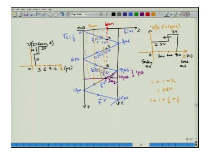
On 1 axis we draw the z axis and down here I will draw the time axis okay so I know what is the length of the or the time delay of the propagation in order to find the time delay I go back to this circuit I know that the length of the transmission line is 900m okay so time delay will be given by 900m and you know that the velocity is 3x 10<sup>8</sup> m/ s so this is about 3 micro seconds okay so what we have 3 micro second, so let us now bill the lattice diagram.
