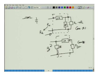
What is the lumped element matching network, it is of course made out of lossless inductances and capacitors okay, you can connect this lossless inductors and capacitors in various forms. We will look at only this particular matching network which is called as the L section matching network. So in the L section matching network we distinguish two cases, one there is a susceptance immediately before the load okay, or immediately after the load I should say.
