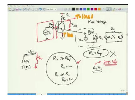
The problem at high frequencies is that in a low frequency condition you might write a simple BJT transistor first not the BJT amplifier you will have some base resistance and some voltage which is what you are amplifying. And then there will be some collector resistance across which you are taking the output right. So this is the VCC for this one and this is the equivalent base resistance that I am writing okay.
