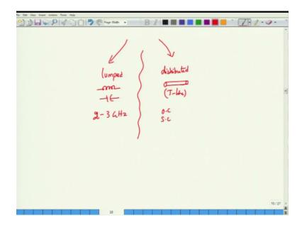
Most matching networks fall into two major criteria one called as the lumped matching networks and the other called as the distributed matching networks. The lumped matching networks utilize the lossless L and C and connect them in appropriate fashion in order to form a matching network at very, very low frequency one can use the transformer for the distributed circuits or for distributed matching networks you actually use the transmission line itself okay.
