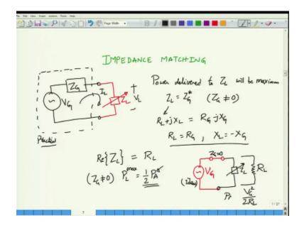
Now if we consider high frequencies we of course also not only at high frequency even at low frequencies we know that the generator impedance or the generator will not necessarily always have an impedance of there, it can also have a reactive component which means that we will be having the complex impedance as an internal impedance something that is not accessible to you. Please remember that this model which I have put inside this dotted lines is actually something of a idealization.
