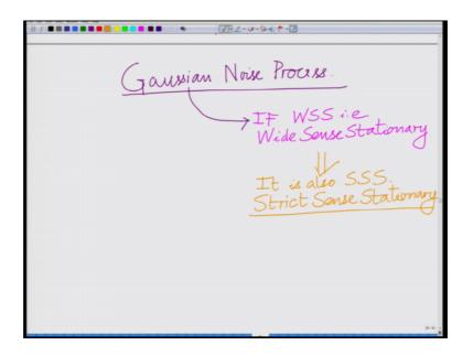
Now, in particular the Gaussian noise process is a very interesting property. If a Gaussian noise process is wide sense stationary, if it is WSS that is if a Gaussian noise process is wide sense stationary then it implies it is also strict sense stationary. Normally this is not true for a random process wide sense stationary random process that is a strict sense
