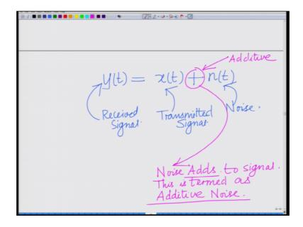
And we have said in that we have looked at a simple system in which y t the received signal y t is simply the transmitted signal x t plus the noise. So, the noise is adding to the transmitted signal x t this is termed as additive noise, alright, we have already seen that this noise which adds to the signal is termed as additive noise.
