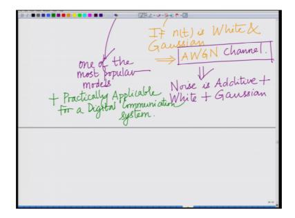
So, the noise is additive in addition if the noise is white and Gaussian this is known as an additive white Gaussian noise channel. One of the most simplest, one of the most frequently used and one of the most popular and also one of the most practically applicable channel models or models for a typical digital communication system.
