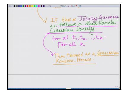
Now, if this joint distribution of noise samples, if this is jointly Gaussian alright. This means it has a multivariate Gaussian density. If this is similar to the scalar Gaussian density, there is a multivariate Gaussian density that is considering multiple random
