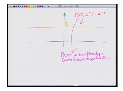
So, you see the PSD is flat power is uniformly distributed overall frequency components similar to white light.
