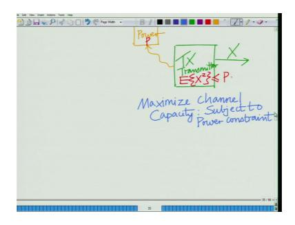
So I have a source or let us say I have a transmitter correct at transmitting a signal X; however, this is basically connected to a power source which supplies the power. So, this transmitter let us say the power is P. So, my transmit power that is has to be limited and remember transmit power is nothing, but the expected value of the X square.
