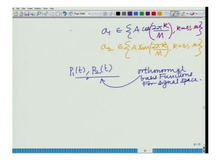
So, this is your transmitted waveform were a 1 belongs to the set A cosine or let us use the index k A cosine 2 pi k by M I am simply changing the index to k, k equal to 0 1 up to M minus 1 and a 1 or a 2 element belongs to A sin 2 pi k by M, k equal to 0 1 up to M minus 1. So, we are transmitting and of course, as we have seen before P 1 t and P 2 t these are orthonormal basis functions for the signal space.
