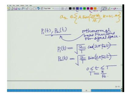
For instance we have said that is a P 1 t equals well again unit norm that is unit energy square root of 2 or T cosine 2 pi F c t, P 2 t is square root of 2 or T sin 2 pi F c t where 0 less than equal to t less than equal to capital T the symbol duration and T correct T equals k over F c or basically contains an integer number of cycles so, that is basically what we have seen before also.
