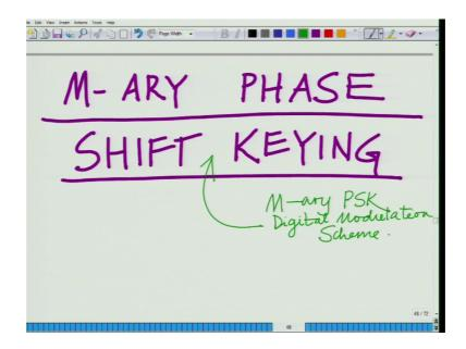
This is another digital modulation scheme and again this also generalizes the concept of binary phase shift keying which has 2 phases.
