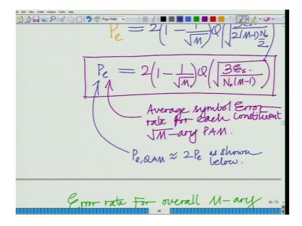
This is a factor of 4 this is twice the probability of probability error of PAM or Pe, QAM approximately twice Pe as shown below.
