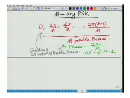
So, we are taking 2 pi 2 pi remember 2 pi corresponds to 360 degrees and we are dividing it into M possible phases. So, by basically what we are doing is dividing 2 pi into M possible phases dividing 2 pi into M possible phases.
