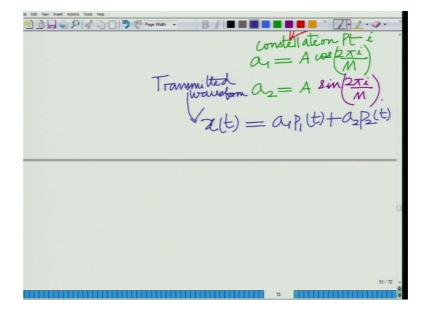
So, the net transmitted waveform x t can be x t equals a 1. So, this is similar to QAM. So, net waveform.
