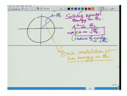
So, a equal to square root of E s that is radius of circle and you can observe that each point has ident each constellation point unlike PAM, each constellation point each constellation point has not only average energy, but each constellation point actually has energy E s. So, that is basically your M-ary PSK constellation.
