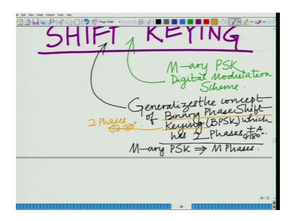
Generalizes the concept of binary phase shift keying BPSK, binary phase shift keying or BPSK which has 2 phases and it generalizes to M-ary phase shift keying. In M-ary phase shift keying basically there are M phases. So, in binary phase shift keying there are 2 phases plus or minus A that is 0 comma 180 degrees. So, if you look at binary phase shift keying there are only 2 phases which are 0 comma 180 degree.
