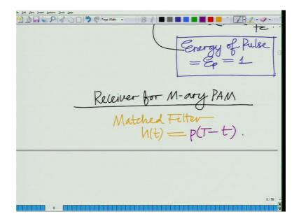
So, receiver operation receiver for M-ary PAM; so obviously, we are again going to use the matched filter. Matched filter h t matched to p t which is equal to that is again the same matched filter maximizes SNR because for the if you go back and look at the derivation of the matched filter, we did not assume any particular modulation we have only assumed a pulse shape, and a symbol a naught a naught need not belong to any particular modulation.
