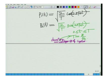
Now unlike FSK We have P 1 t equals square root of 2 over t, cosine 2 pi f c t and P 2 t, equals square root of 2 pi f c 2 over t sin 2 pi f ct both for 0 less than equal to t less than equal to t. And t equals k over f c that is the duration spans an integer number of cycles. This is we have seen several times before that is duration equals and integer number of cycles.
