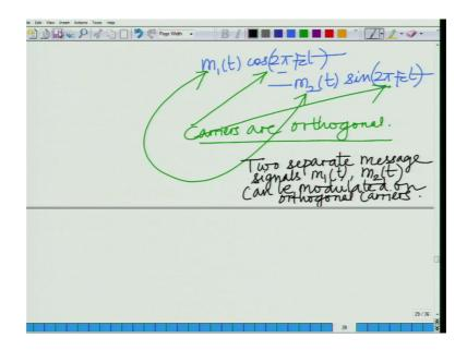
So, 2 different message signals can be modulated one on cosine and one on sin because these 2 are orthogonal. So, these 2 carriers are orthogonal we have seen in quadrature carrier multiplexing that these 2 carriers or orthogonal therefore, you can modulate 2 separate signals 2 separate signals message signals m 1 t, comma m 2 t can be modulated on.
