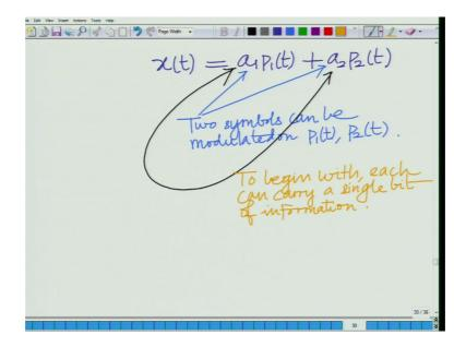
Now, is basically I am going to generate my signal x t as a 1 times P 1 t plus a 2 times P 2 t. Now, note is that I am modulating not one symbol, but 2 symbols a 1 and a 2. So, 2 symbols or 2 bit is can be modulated on P 1 t and P 2 t. For instance, each can carry one bit of information they can more also, but to begin with let us say each carries to begin with let us say, to begin with let us say each can carry a single bit of information.
