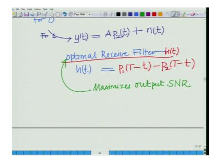
We have seen the matched filter optimal received filter, optimal receive filter a is h t equals P 1 well T minus t minus P 2 T minus P 2 T minus t. So, this is the optimal receive filter, optimal receive filter in the sense we must be well familiar by now optimal in the sense this maximizes the output SNR or signal donates power ratio.
