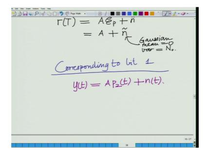
So, basically the output is r T equals well A E p plus n tilde setting E p equal to 1 this is a times writing E p again because it is. So, that the expression is general and can be valid also for scenarios where E p is not necessarily equal to 1 n tilde this is Gaussian with mean equal to 0, and variance is equal to n naught. Now similarly corresponding to the transmission of information bit corresponding to bit 1, well corresponding to bit one we have y t equals a times P 2 T plus n t.
