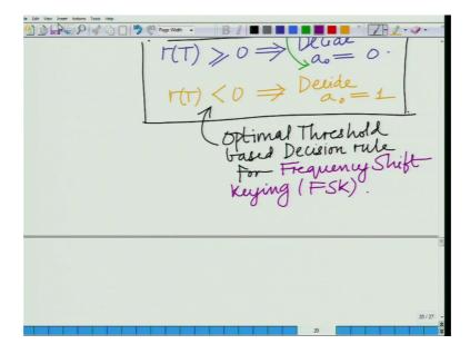
This is the optimal decision of FSK is not very different from that. In fact, very similar to that of b s k this is the optimal. In fact, we can say threshold based decision rule for frequency shift keying FSK or frequency shift keying, that is f frequency shift keying FSK.
