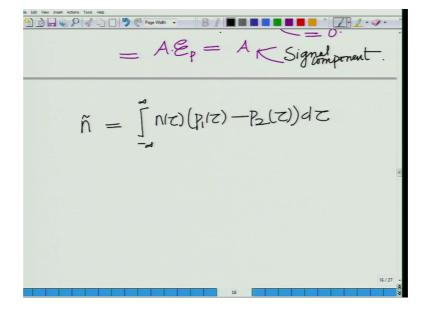
Therefore all that is left is a times E p substituting E p equal to 1, this is remember the signal component after matched filtering. Now if you look at the noise component n tilde, which is equal to minus infinity to infinity n tau P 1 tau minus P 2 tau d tau.
