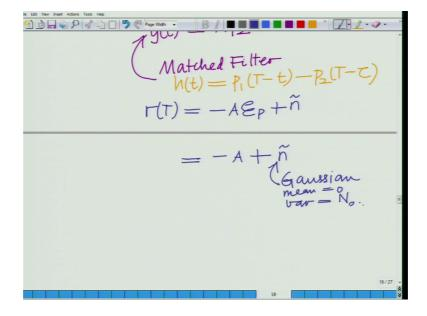
Now, when we matched filter this, or receive filter this, with once again h of t equals P 1 T minus t minus, P 2 T minus t the output will be well, you can verify this r T is minus A E p plus n tilde again setting equal to 1, this is equal to minus A E p or minus simply a minus A plus n tilde, where n tilde is Gaussian. Once again is a same thing the mean equal 0 the variance is equal to n naught.
