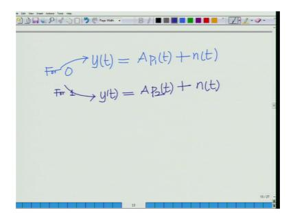
So, we are considering 2 different frequencies f 1 and f 2 since they are wave forms are shifted versions of each other with frequencies this is known as frequency shift key all right. And what we have seen in this is that my y t corresponding to 0 is a times P 1 T plus n t. That is, this is for information bit 0 for 1, we have y t equals a times P 2 T plus n t.
