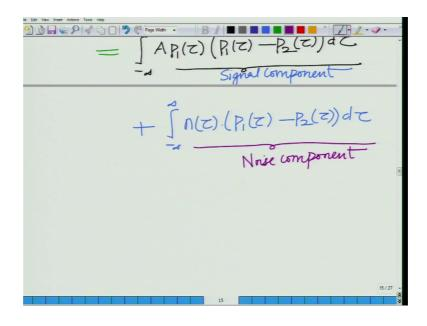
So, corresponding to the transmission of information signal the inform corresponding to information bit 0, we have computed what is the output after filtering with h t followed by sampling at t equal to capital T where capital T is the symbol duration these are in the signal component and the noise component.
