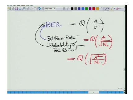
And the corresponding bit error rate again we can see, corresponding bit error rate there is if you look at this bit error rate, which is either which is again another thing that you should be familiar very familiar with, by now this is the bit error rate bit error probability or this known by many terms or the probability, this is equal to Q times A divided by sigma which is equal to Q times A divided by square root of n naught, which is equal to Q times A square divided by n naught.
