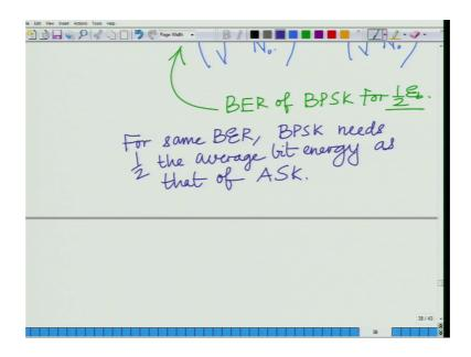
So, if you look at this for same bit error rate for an identical bit error rate, for the same bit error rate BPSK half the average bit energy as that of amplitude shift keying which implies that energy per bit of BPSK equals half energy per bit of amplitude shift keying.
