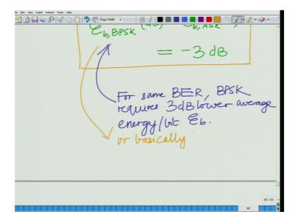
So, in dB terms for same BER BPSK lower average energy per bit or in other words or basically ASK amplitude shift keying 3 dB higher E b when compared to when compare to or basically amplitude shift keying requires 3 dB higher E b when compare to BPSK for the same bit error rate. So, that is the interesting observation that we would like to maintain.
