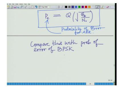
So, this is the probability of error for amplitude shift keying. This is the probability of error for amplitude shift keying. Now compare this with probability of error of binary phase shift keying compare it with probability of error of binary phase shift keying which is equal to q, remember this is Q square root of 2 E b over N naught this is the probability of error of binary phase shift keying.
