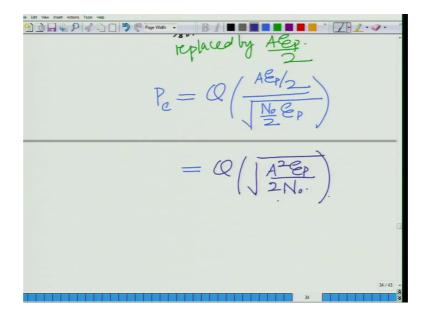
Therefore, probability of error is Q A E p divided by 2 A E p divided by 2, divided by square root of n naught by 2 times E p, now, we are going to substitute which is equal to well let me first simplify this, which is equal to Q square root of A square E p by N naught which is equal to Q A square E p by 2 N naught.
