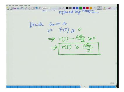
Hence the optimal detector again can be to decide a naught equals A if r tilde T greater than or equal to well 0 implies r T minus A E p by 2 greater than equal to 0 implies r T greater than or equal to A E p by 2.
