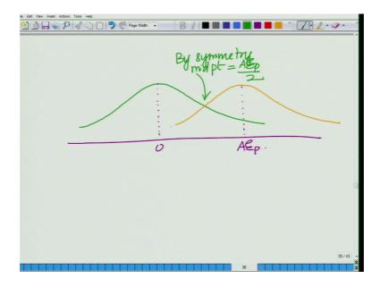
But in amplitude shift keying corresponding to a naught equal 0 the mean is still 0 correct and corresponding to this amplitude corresponding to a naught equals A the
