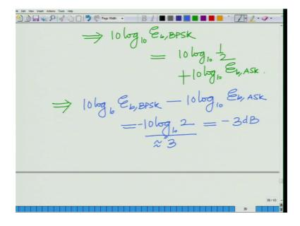
Which implies that the dB difference between the average bit energy of BPSK and ASK is 10 log to the base 10 that is the dB difference minus 10 log to the base 10 energy per bit ASK equals minus 10, equals minus 10 log to the base 10 2; 10 log to the base 10 of 2 is 3 this quantity is approximately 3 which means this is minus 3 dB.
