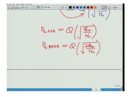
So, for amplitude phase amplitude shift keying it is equal to Q square root E b over N naught for binary phase shift keying probability of error, for binary phase shift keying is
