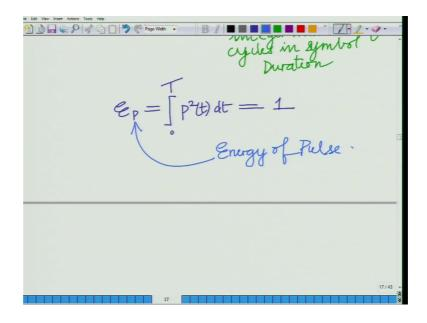
And we have already seen that energy of the pulse if you look at integral 0 to T, P square t that is energy of the pulse previously in binary phase shift keying, we have used the similar pulse we have seen that energy of the pulse, energy of the pulse is unity. We have already seen this.
