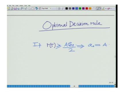
So, the optimal decision rule is not to compare r T with 0, but to compare r T with this threshold A E p divided by 2 which E p is 1. So, this is a by 2. If r T is greater than or equal to A E p divided by 2 implies, this implies the decision is a naught equal to A.
