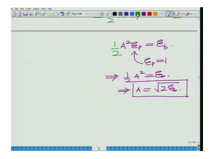
Now, given the average bit energy is E b, we need to have half a square E p is equal to E b or is equal to E b. Further we have E p equals one because of pulse is normalized to unity power which implies half A square is equal to E b which implies or which rather
