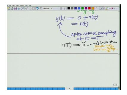
Now, therefore, what is r T therefore, y t is simply 0 plus n t equals n t. After matched filtering and sample with p sampling at t equal to T after M F and sampling at t equal to capital T what we get is r T is simply because there is no signal component there is only going to be the noise which is n tilde. Once again n tilde nothing changes n tilde is Gaussian with mean equal to 0, variance equals n naught by 2 times E p.
