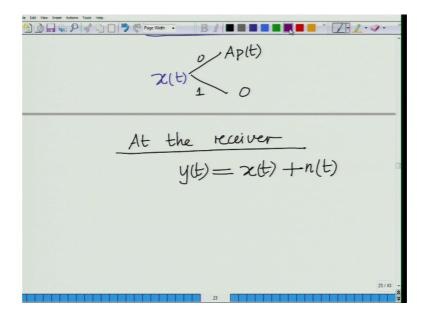
So, remember we are transmitting x t is either A times p t corresponding to information bit 0 or it is equal to 0 corresponding to information bit 1. At the receiver we have, at the receiver we have y t - y t equals x t plus n t where what is n t, we have already seen what is n t.
