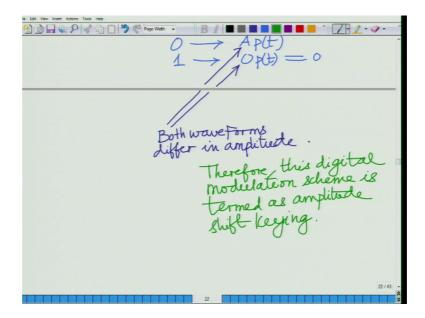
Now, as I have already told you here we have 0 being mapped to A times p t and formally stating this once again 1 is mapped to 0 times p t equals 0. Both the schemes differ in amplitude that is if you look at both the schemes both the waveforms differ in amplitude. Therefore, this digital modulation scheme is termed therefore; this digital modulation scheme is termed as amplitude shift keying. So, that is basically amplitude shift keying or ASK; amplitude shift keying or ASK.
