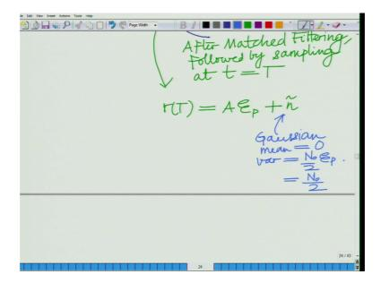
I am using a lot of results from what you have derive before for the general optimal received processing and binary phase shift keying scenario. So, n tilde is Gaussian with mean equal to 0 variance equals N naught by 2 times E p, but E p equals 1, so you can also say this is equal to N naught by 2.
