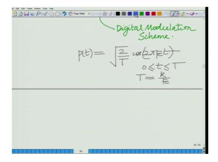
And in amplitude shift keying. So, this is another as we have already said this is another yet another digital modulation scheme, this is yet another digital modulation scheme in which we employ the pulse shape p t equals square root, again a similar pulse shape square root 2 pi f c cosine t for 0 less than equal to t a less than equal to capital T where capital T is the symbol duration and T equals k over F c.
