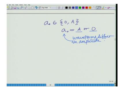
So, the symbol a naught belongs to the set 0 comma A. So, a naught equals either A or 0. So, there is difference, waveforms differ in waveforms differ in the amplitude. So, a naught can be either A or 0.
