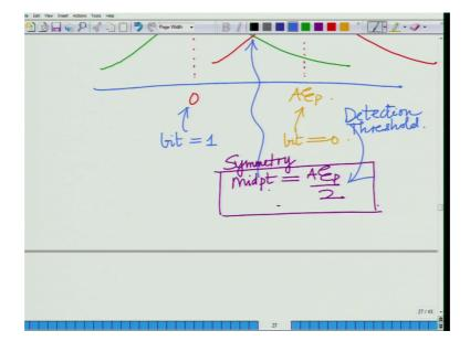
So, this is the Gaussian corresponding to bit 1, this is the Gaussian for bit equal to 0 by symmetry the midpoint is A E p divided by 2 which is the detection threshold which is
