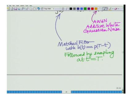
N t is basically well n t is additive, Additive White Gaussian Noise this is AWGN or this is Additive White Gaussian Noise. Now what is optimal processing at the receiver? Optimal processing at the receiver is we have to matched filter, we matched filter h t, matched filter with h t equals p T minus t that is matched filter followed by sampling at t equal to T, followed by sampling at t equal to T.
