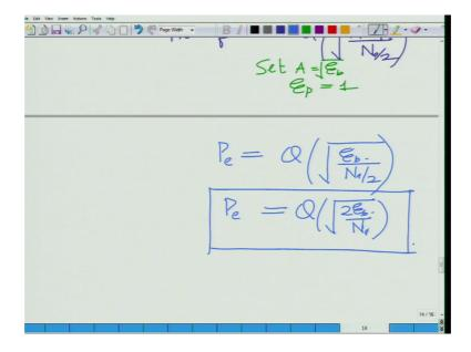
And therefore, probability of error if I denoted by P E is equal to Q square root of A square is E b over N naught by 2 which is equal to Q square root of 2 E b over N naught that is your P E which is the probability of error of this binary phase shift key system.
