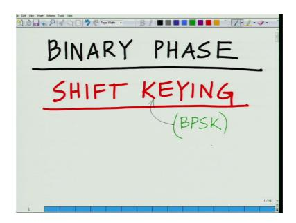
So, what I want to start looking at is a different modulation scheme which is termed as binary phase shift keying also termed as also we can call this a also abbreviated as rather BPSK; this is abbreviated as BPSK and this is basically it is a digital modulation scheme its one of the several schemes for digital modulation.
