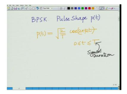
Now, what happens in by BPSK the pulse shape in BPSK the pulse shape or simply you can call this the pulse remember every digital communication system employs a pulse or a pulse shaping filter; the response of the pulse is given as well P T equals square root 2 over T; correct, square root 2 over T cosine 2 pi F c t such for 0 less than equal to t less
