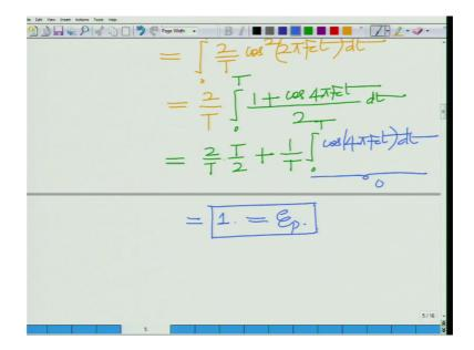
Well integral 0 to T 1 plus cosine 4 pi F c t divided by 2 d t which is equal to well 2 over T times t over 2 plus 1 over T times integral 0 to t cosine 4 pi F c t d t and you know this quantity or rather this integral this integral is 0 therefore, what is left is 2 over T times t over 2 equals 1 which is equal to your E P.
