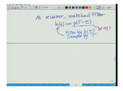
So, we know the match filter match filter is given for this the match filter at receiver match filter is h t equals P T minus tau that is filter with h t optimal processing is filter by h t followed by sample at capital T sample by t and now you are wondering why we are using this P capital T minus tau that also probably is worth clarifying because rather than using simply P minus T why are we shifting it by capital T.
