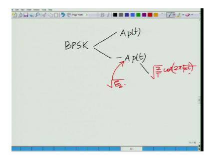
So, in this BPSK we are employing 2 waveforms a times or a naught times or let us put it this way a times P t A times P t minus; A times P t, the only thing is that P T equals square root of 2 over T cosine 2 pi F c t and a is square root of E b.
