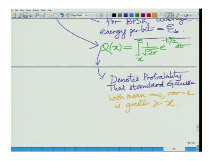
This is the probability it denotes the probability that denotes the probability that standard Gaussian with mean equal to 0 variance equal to one is greater than or equal to x that is basically what this is x that is
