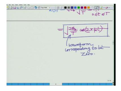
Which is equal to again square root of 2 E b over T cosine 2 pi F c t, this is the wave form corresponding to 0, this is the wave form just to summarize this once again although it should be very clear this is the wave form corresponding to this is the wave form corresponding to bits 0, this is the waveform corresponding to bit 0.
