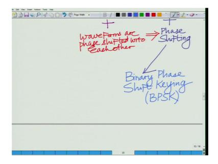
So, the motivation behind this calling this binary phase shift keying is basically there are binary waveforms 2 waveforms which are phase shifted with respect to each other therefore, this is known as binary phase shift keying and now we know what is optimal now we know this is what is. So, we are employing 8 A times P T minus A times P T we already see the similar scheme for instance.
