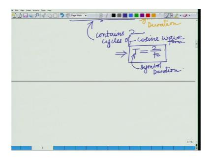
This contains basically contains 2 cycles contains 2 cycles of the cosine waveform implies T equals 2 over F c on over F c is the period. So, symbol duration is basically that is symbol duration equals 2 over F c. So, this is the symbol duration symbol duration equals 2 over F c.
