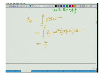
What is the meaning of that if we compute E P energy of the pulse that is minus infinity to infinity minus infinity to infinity P square t d t that is equal to well 0 to capital T 2 over T cosine square 2 pi F c t d t which is equal to 2 over T.
