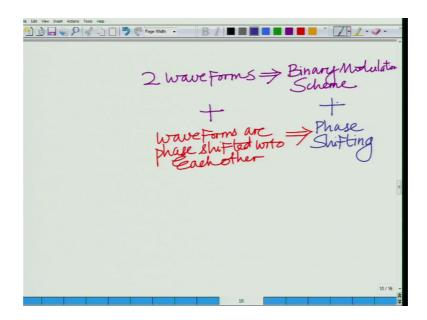
So, basic is, so basically again we have 2 waveforms implies this modulation scheme is a binary modulation scheme plus waveforms are phase shifted with respect to each other.
