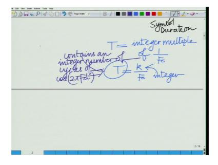
And further correct, we have this condition that T is an integer multiple of 1 over F c that is T equals k over F c where k is a integer; where k is a; this is a integer that is basically this duration T symbol duration contains an integer number of cycles of cosine 2 pi F c t and contains an integer number of cycles of cosine 2 pi F c t.
