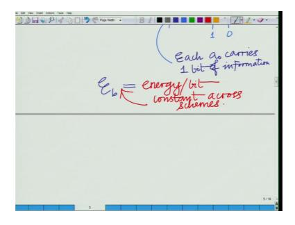
So, we are going to denote this quantity by E b; E b equals the energy per bit and this we are going to hold constant across this we are going to hold constant across the schemes.
