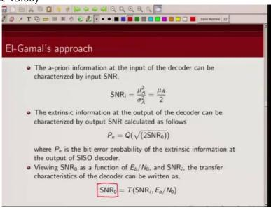
in terms of input S N R and our operating signal to noise ratio. So what we can do is we can view the output S N R of the extrinsic
