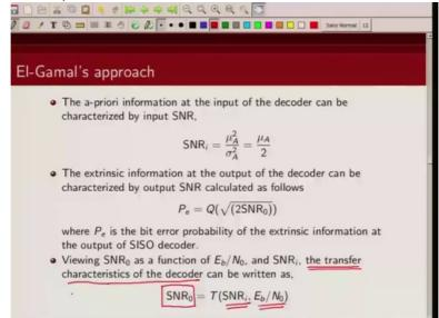
view it as a function of input S N R of a priori values as well as channel, operating channel signal to noise ratio. So this relation characterizes how my decoder will behave. Because remember with iteration your extrinsic information is changing as a function of
