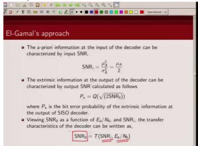
this is crucial, so this is basically what I call the transfer characteristics of the decoder. Because my decoder is a function of
