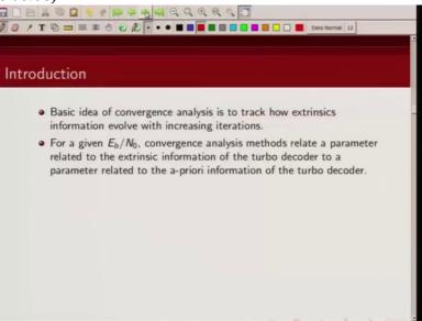
evolving? So what we do is, for a fixed signal to noise ratio we have a set of received values. So what we do is we try to relate a parameter which is related to the extrinsic information of the turbo decoder and
