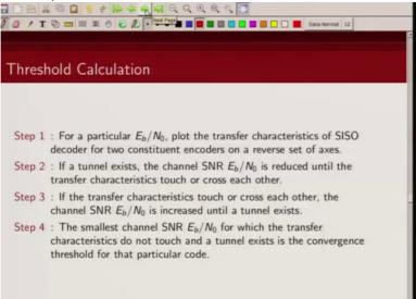
So the smallest channel S N R for which these two transfer characteristics which have been plotted on reverse axes, they do not touch and a tunnel exist is basically the convergence threshold for that particular code. So that would give the S N R, minimum S N R under which that particular code will converge and it will have a
