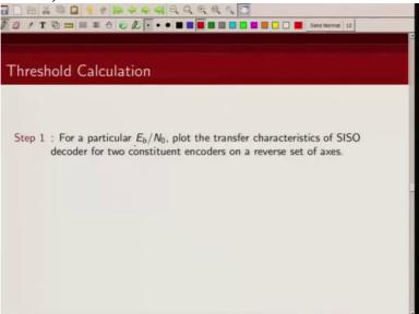
particular signal to noise ratio, we plot the transfer characteristics of this soft input soft output decoder. We plot them on reverse set of axes. Now what do I mean by reverse set of axes? So for the first, my S N R in is on x axis, and
