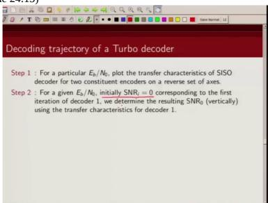
the resulting output S N R which we look vertically for using the transfer characteristics for decoder 1.
