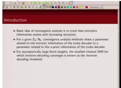
And for an asymptotically large block size the smallest channel S N R for which iterative decoding algorithm converges is known as decoding threshold. So this iterative
