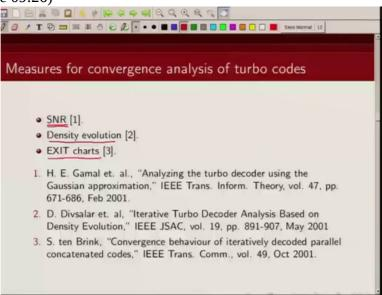
observe how, with iteration your extrinsic information is growing. And these are the three references, the first one corresponding to this S N R technique, the second one corresponding to this density evolution technique and third corresponds to this EXIT chart technique.
