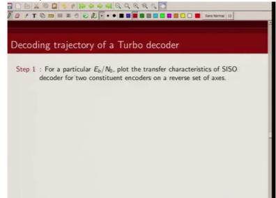
what we do is for a particular signal to noise ratio as I said, we plot these transfer characteristics of two constituent encoders on reverse set of axes. So for decoder 1, S N R in will be on
