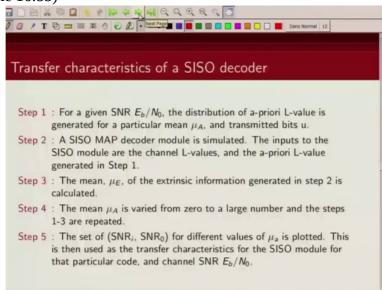
And finally what we do, we plot this input output relation for a particular channel S N R. So this is my input a priori S N R, this is the extrinsic information S N R. We plot it for a particular value of signal to noise ratio and this is my transfer characteristic for that particular decoder
