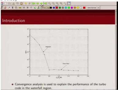
So this is a typical performance of a turbo code. If we take a larger block size, this is for a block size, I think 65000 plus, so if you take a large block size, this is typical performance of a turbo code. On x axis, I have signal to noise ratio and on the y axis, I have plotted
