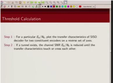
Now if these transfer characteristics do not cross, there is a tunnel in the sense they do not touch each other, then what we do is the channel, operating channel S N R is reduced until these transfer characteristics just about touch.
