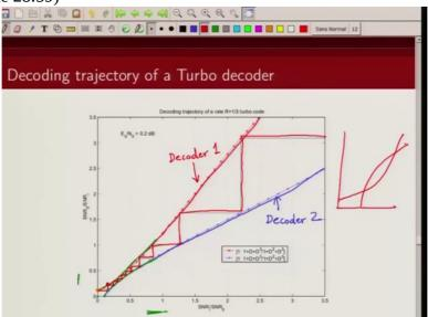
let's draw the decoding. So this is transfer characteristics of decoder 1
