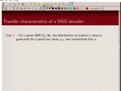
So then how do we draw the transfer characteristics? For a given signal to noise ratio, the distribution of a priori L values is generated for a particular mean mu a and transmitted bit u. How?
