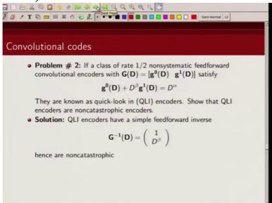
quick look-in encoders have a very simple encoder inverse, a feed forward encoder inverse and that is given by this. You can verify that G D G D inverse is your d times alpha,
