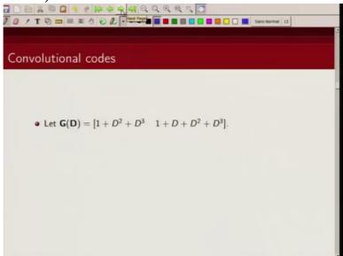
take an example where feed forward inverse exists. So we are considering a feed forward rate 1 by 2. This is a rate 1 by 2 encoder.
