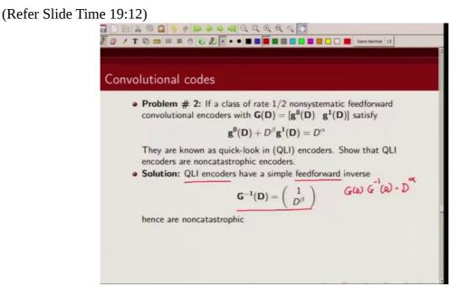
Ok. Now note that the encoder inverse of quick look-in encoder has just 2 tabs, 1 and this d beta. And it has a feed forward inverse so it cannot be a catastrophic encoder. We just showed in the previous slide that
