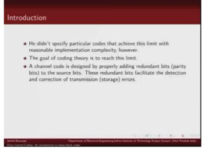
did not specify how to design such code; so basically where coding theories come into picture. So how do we design an error correcting code? An error correcting code is designed by adding some redundant bits to the message bits. Message bits, we call them information bits and those additional redundant bits that we add, those are known as parity bits. So error correcting code is designed by properly adding some redundant bits to your message bit and
