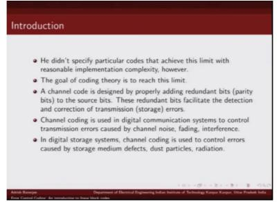
in digital storage system you want to correct the error caused due to storage media defect, dust particles, radiations we use error correcting codes there.
