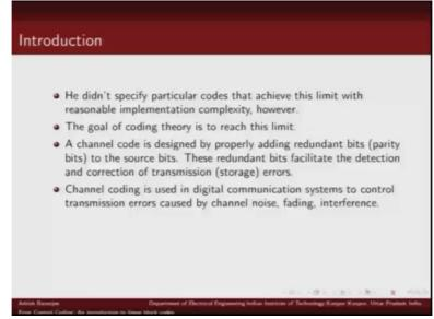
code has wide range of applications in digital communications and storage. I have listed few of the uses, for example when we send a signal over communication link; it gets corrupted by noise, fading, interference. So to combat the interference of all these basically we use the error correcting codes to correct the errors. Similarly
