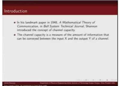
capacity is defined as the maximum amount of information that can be conveyed from the input to the output of a channel. Shannon
