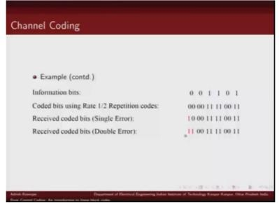
1 1 is a valid code word for 1; the decoder is not able to detect this error. So this rate one half repetition is able to detect single error but it is not able to detect double errors.
