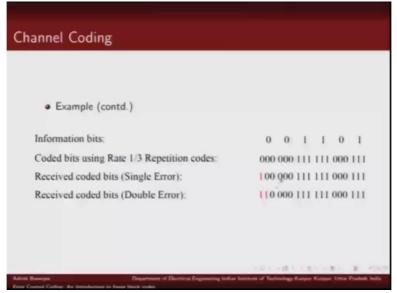
If we look at other sets of bits 0 0 0, there is no error here; 1 1 1 no error, again no error here, no error here. So rate one half repetition code was able to detect single error, even rate one third code is also able to detect single error.
