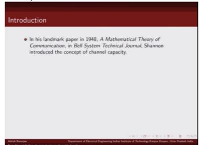
So in his landmark paper in 1948, Shannon introduced this concept of channel capacity, that what is the maximum rate at which we can communicate
