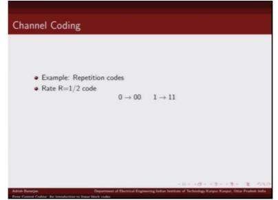
So the rate is defined as the ratio of number of information bits to number of coded bits. So when I say rate one half code, I mean there is one information bit or one message bit and there are two coded bits.
